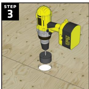
Drill a 2 ½" hole for the drain pipe using the transferred marks and have a qualified plumber install a 2" ABS drain pipe. The drain pipe should be installed so that the top of the pipe is 1 ⅜" below the top of the shower area sub-floor.
