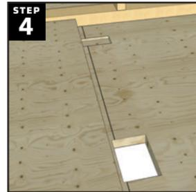
Using appropriate tools (e.g. router), cut the end cap recesses a minimum of 3/16" deep. Cut out the 4" x 6" center drain opening completely.
