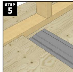
If the linear drain body is wider than the shower opening, it must be rough cut to fit so that it can be placed inside the shower opening.
