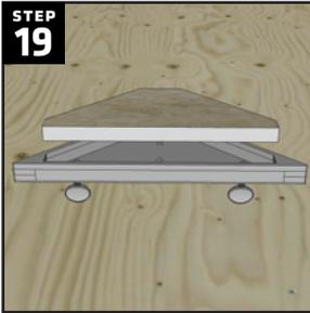
Install the cut tile into the drain access cover using a small amount of thinset or joint sealant. Use the provided set screws to raise or lower the tile so that the top surface is flush with the top of the drain cover.
